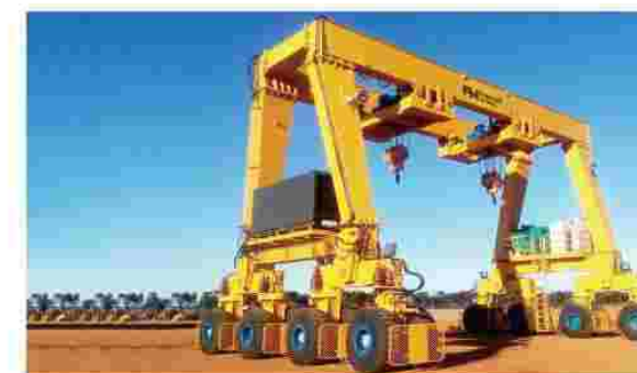
► Double wheel double girder gantry crane
